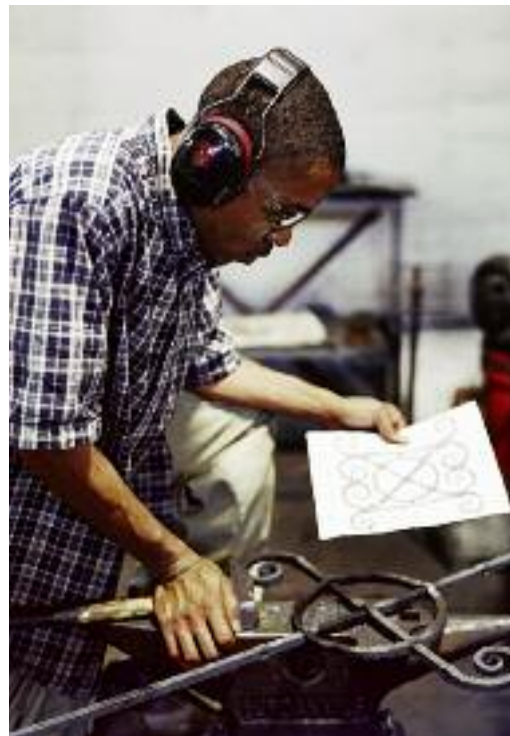
Julian Williams consults his sketch as he works on a hand-forged window grill, following in the footsteps of Philip Simmons, the Charleston craftsman who for more than 75 years enhanced the city's collection of decorative ironwork.
